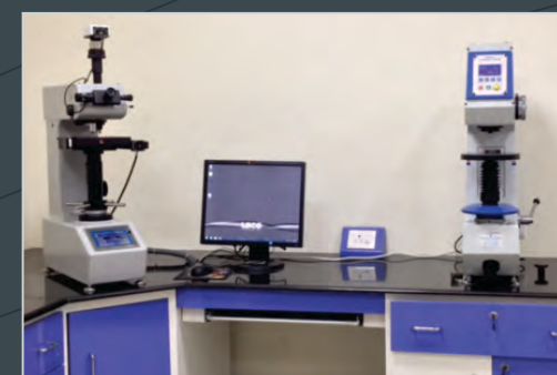
Vickers Micro and Macro Hardness plus Rockwell Superficial Hardness Testers
