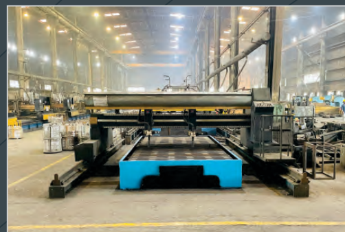
CNC Controlled PTA wear plate machine
