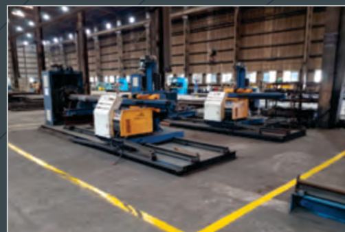
Battery of pipe welders
