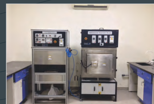
ASTM Dry Abrasion and Air jet Erosion Test Rigs until 800 deg C
