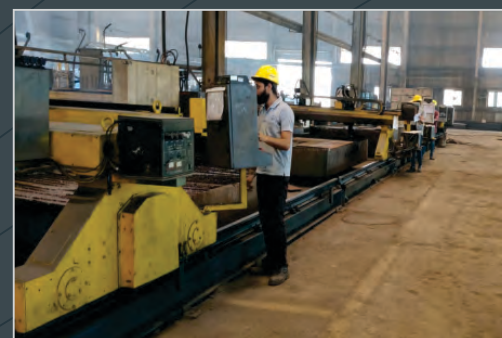
Battery of CNC controlled cutting machines
